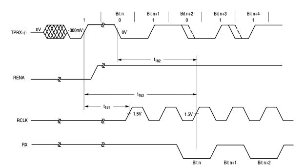
Figure 32. TPRX Receive Timing (Start of Frame)
