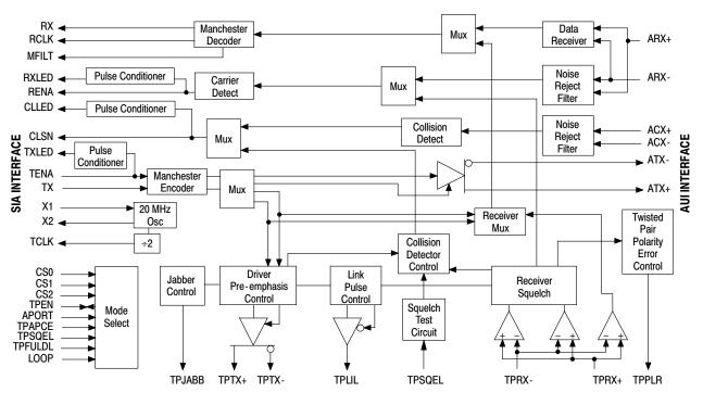
Figure 1. 10Base-T Interface Block Diagram
