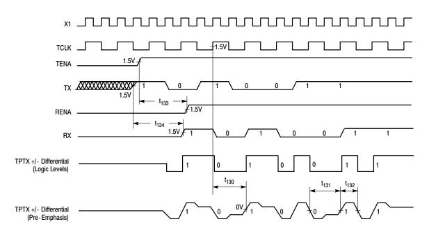
Figure 25. TPTX Transmit Timing (End of Frame) Switching
