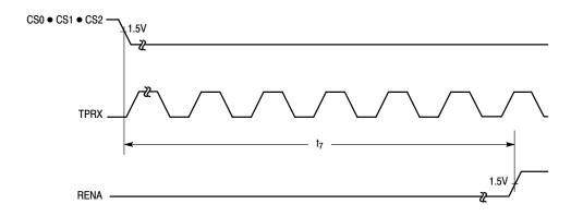
NOTE: CS0 • CS1 • CS2 is the logical AND operation and refers to the pins not at Logic 1.
