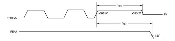
Figure 34. TP Receive Link Integrity Switching
