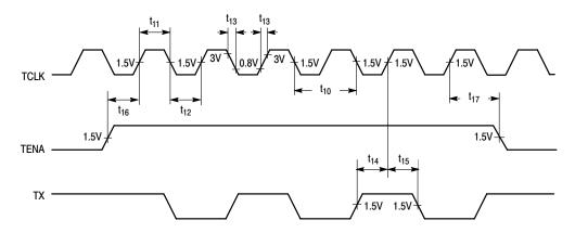
Figure 11. Receive Timing (Motorola Start of Frame)
