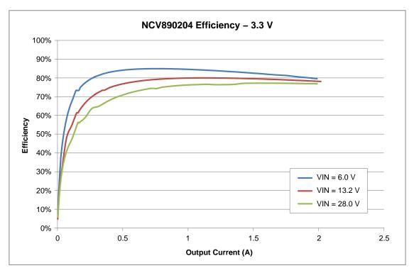
Figure 8. Efficiency with a 3.3 V Output
