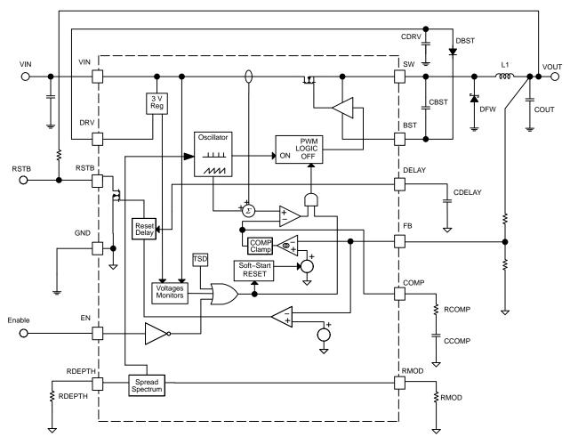
Figure 2. NCV890204 Block Diagram
