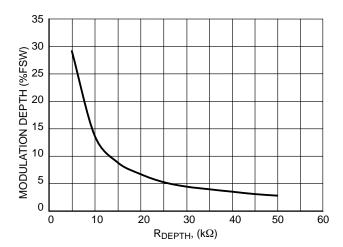
Figure 7. Modulation Depth vs. RDEPTH Value
