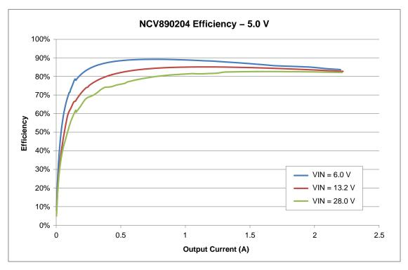
Figure 9. Efficiency with a 5.0 V Output
