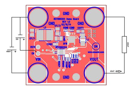
Figure 5. NCV890204 Board Connections
