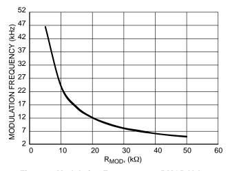
Figure 6. Modulation Frequency vs. RMOD Value
