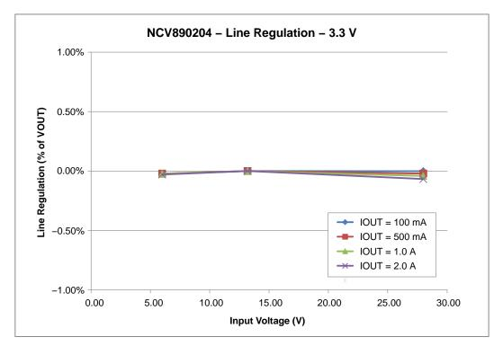
Figure 10. Line Regulation for a 3.3 V Output
