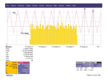
The modulation depth and modulation frequency are each set by an external resistor to GND. The modulation frequency can be set from 5 kHz up to 50 kHz using a resistor from the RMOD pin to GND. The modulation depth can be set from 3% up to 30% of the nominal switching frequency using a resistor from the RDEPTH pin to GND. Please see the curves below for typical values:
