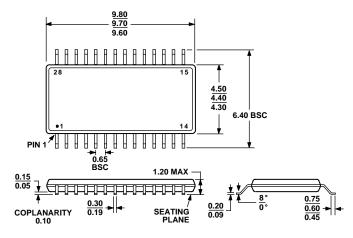
COMPLIANT TO JEDEC STANDARDS MO-153-AE Figure 8. 28-Lead Thin Shrink Small Outline Package [TSSOP] (RU-28) Dimensions shown in millimeters
