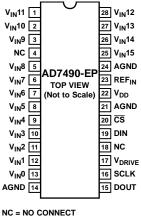
NC = NO CONNECT ALL NC PINS SHOULD BE CONNECTED STRAIGHT TO AGND
