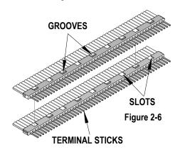
Repeat step 5 for the remaining LFH™ terminal sticks in the connector. The groove orientation on the terminal sticks must be the same for all the sticks; if it is not, the sticks will not stack properly. See Figure 2-7.
