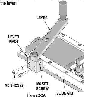
1. Remove the two M6 SHCS from the lever pivot mounted to the side gib. See Figure 2-2A.
