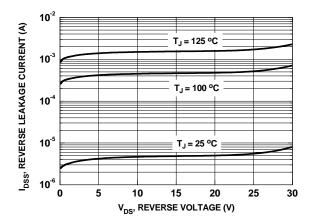
Figure 15. SyncFET<sup>TM</sup> body diode reverse leakage versus drain-source voltage
