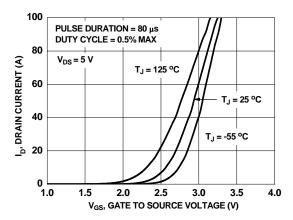
Figure 5. Transfer Characteristics
