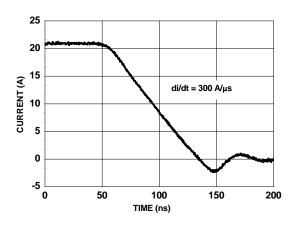
Figure 14. FDMS0309AS SyncFET<sup>TM</sup> body diode reverse recovery characteristic
