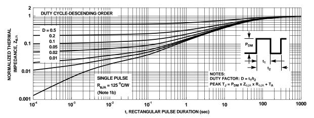
Figure 13. Junction-to-Ambient Transient Thermal Response Curve
