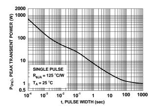
Figure 12. Single Pulse Maximum Power Dissipation
