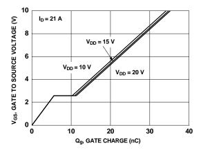
Figure 7. Gate Charge Characteristics
