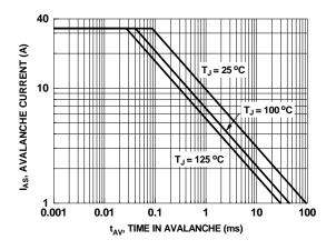
Figure 9. Unclamped Inductive Switching Capability
