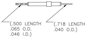
3. TIP IS REVERSIBLE: LOOSEN AND REMOVE NUT TO ACCESS TIP.
