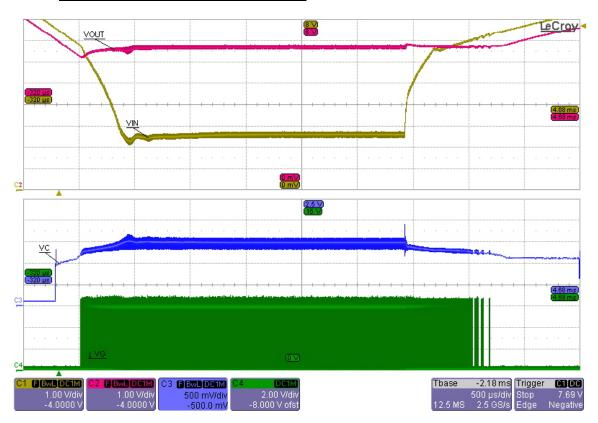
Figure 3 NCV887801 Demo Board Waveforms
