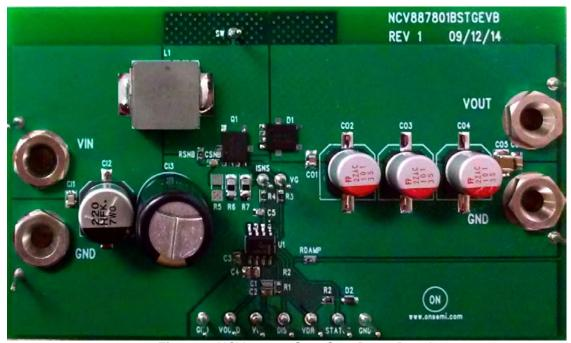
Figure 1. NCV887801 Start-Stop Demo Board
