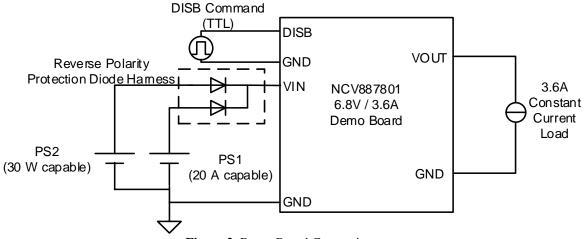
Figure 2. Demo Board Connections
