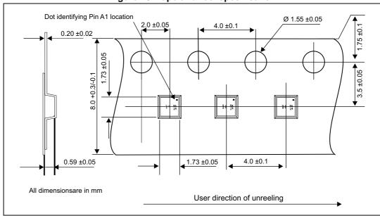
Figure 13. Tape and reel specification
