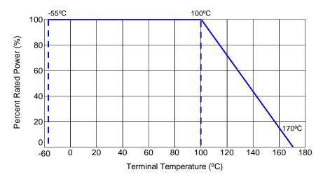
Operating temperature range of -55 to 170°C. Storage condition: 5~35°C, humidity of 40~75%.
