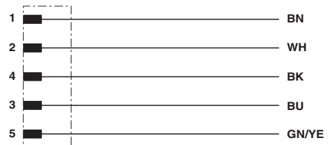
Contact assignment of the M12 plug
