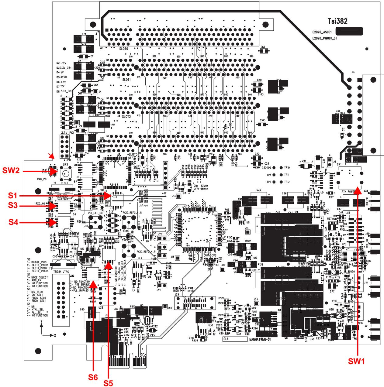
Switch S1 is used to manually set PCI bus modes.
