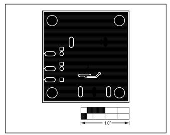
Figure 4. MAX15062B EV Kit PCB Layout—Solder Side
