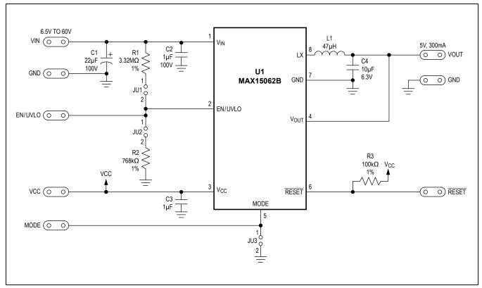
Figure 1. MAX15062B EV Kit Schematic
