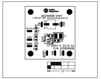
Figure 2. MAX15062B EV Kit Component Placement Guide—Component Side
