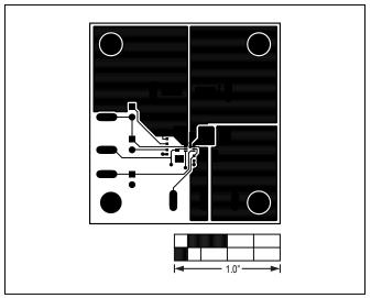
Figure 3. MAX15062B EV Kit PCB Layout—Component Side
