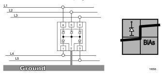
b. If symmetrical clamping behaviour is required the VESD05A5A-HSF can also be used as a bidirectional symmetrical protection device protecting up to 4 lines. In this case pin no. 2 must not be connected.
