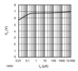
Fig. 5 - Typical Reverse Voltage  $V_{\text{R}}$  vs. Reverse Current  $I_{\text{R}}$
