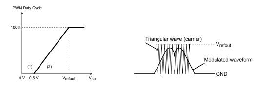
Note: An amplitude of the modulated waveform becomes maximum when  $V_{SP} = V_{refout}$ . The PWM duty cycle that is obtained with the  $V_{SP}$  voltage of  $V_{refout}$  is defined as 100%.
