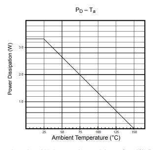
Measured on a board (140 mm  $\times$  70 mm  $\times$  1.6 mm, Cu: 50%) Rth (j-a) = 38°C/W
