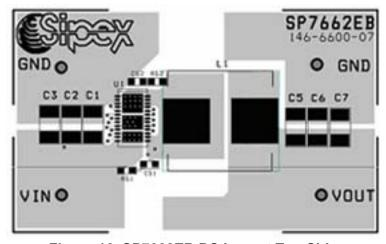
Figure 16. SP7662EB PC Layout Top Side
