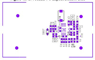
Figure 20. SP7662EB PC Layout Bottom Side Components
