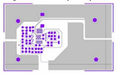
Figure 19. SP7662EB PC Layout Bottom Side
