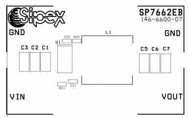
Figure 15. SP7662EB Component Placement
