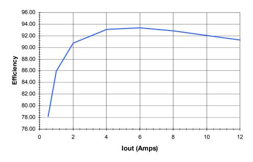
Figure 1. Efficiency vs Load
