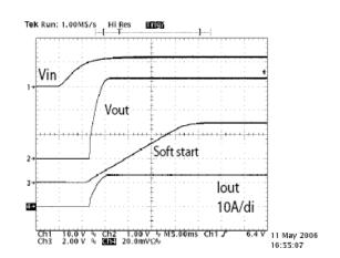
Figure 6. Output load Short Circuit
