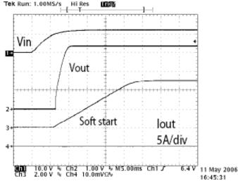
Figure 8. Startup into no load
