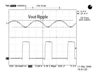
Figure 2. LX node output ripple voltage
