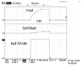
Figure 4. Load Step Response 0->12A
